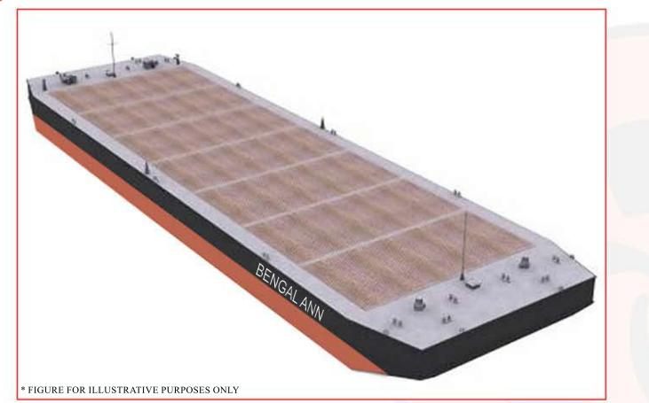
LENGTH : 54.86 m (180.00 ft) BREADTH : 18.29 m (60.00 ft) DEPTH : 3.66 m (12.00 ft) DRAFT (EMPTY) : 0.60 m (1.97 ft) DRAFT (MAX) : 3.20 m (10.50 ft) DWT : 2,400 T DECK STRENGTH : 15 T / m<sup>2</sup> GRT : 914 T NRT : 274 T CLASS: RINA PLACE / YEAR OF BUILD : INDONESIA / 2021 FLAG : U.A.E. OTHERS : NAVIGATION LIGHTS, TOWING BRIDLE, BLACK DIAMOND
